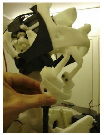
Leaving the head up, Slide the jaw assembly in to the head.
