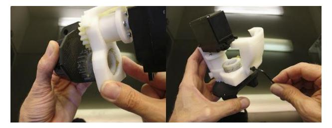
Mount this assembly to the assembly "MainGear" and "NeckHinge" using some grease to ease the rotation. "GearHolder" should be aligned with "NeckHinge" and your servo should be still at 90°.
