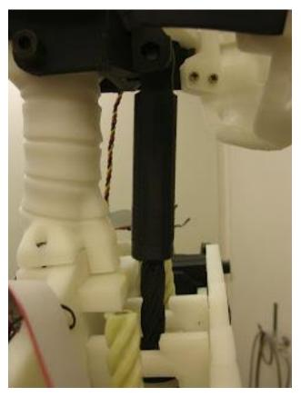
Fix "NeckHinge" to "Neck" with a 8mm bolt (or print one from the hand). Assuming you have already fixed your HS-805BB servo in the Torso assembly.
