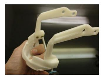
Screw "Jawsupport" to "Jaw". Make sure the flat surfaces of the "Jawsupport" are on the inside.
