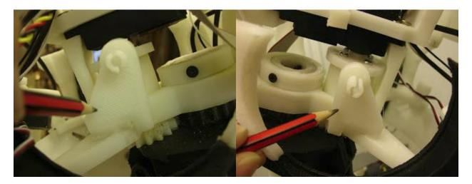
Glue the two "JawHolders" on both sides of whole assembly with acetone. It comes/fit on the "FaceHolders".
