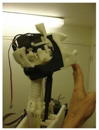
Now the whole head should be able to go up and down if the servo turns from 0 to 180. Make a test with the arduino. Run this test carefully.
