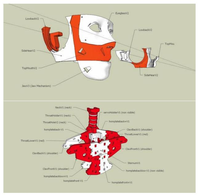
Double check that you have all the materials necessary BEFORE continuing. Note that when affixing "SideHearV2" on the face, you MUST glue this piece to its neighboring pieces AFTER you have assembled the internals of the head. Otherwise, you have no way of accessing the inside parts.
