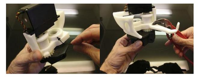
Screw "Ring" to "MainGear". Try to avoid slack between parts.
